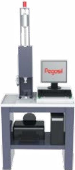
Falling mass shock absorption tester
