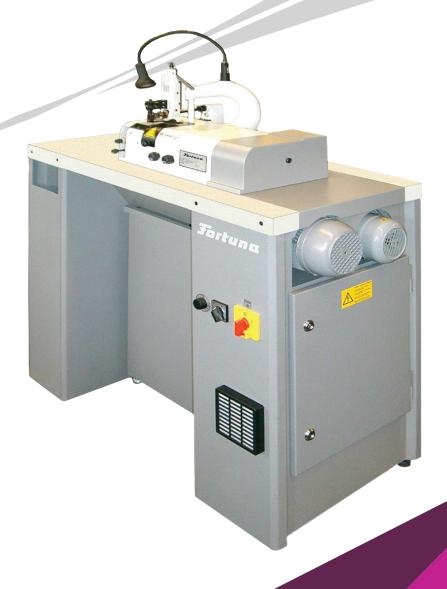
Maximum working width: 50 mm. Used for production purposes in the rubber and plastics industries..
